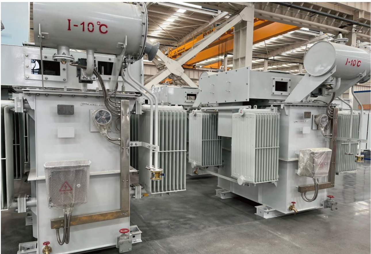
33kv-3150kvaOil immersed transformer
