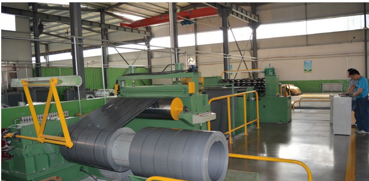
Silicon steel sheet crosscutting machine
