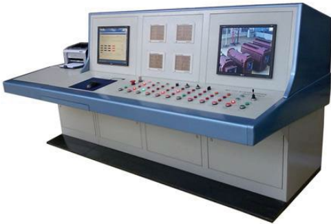
Comprehensive experimental platform for power transformer
