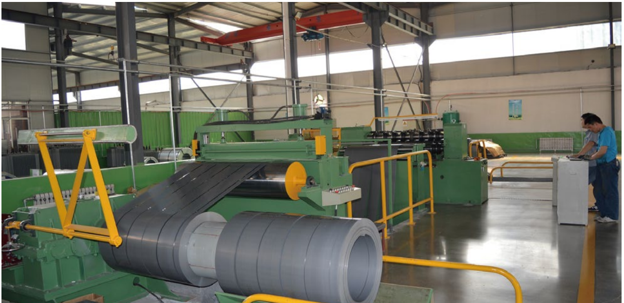
Silicon steel sheet crosscutting machine
