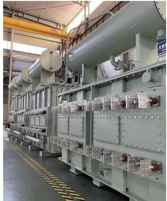
>35kV furnace transformer
