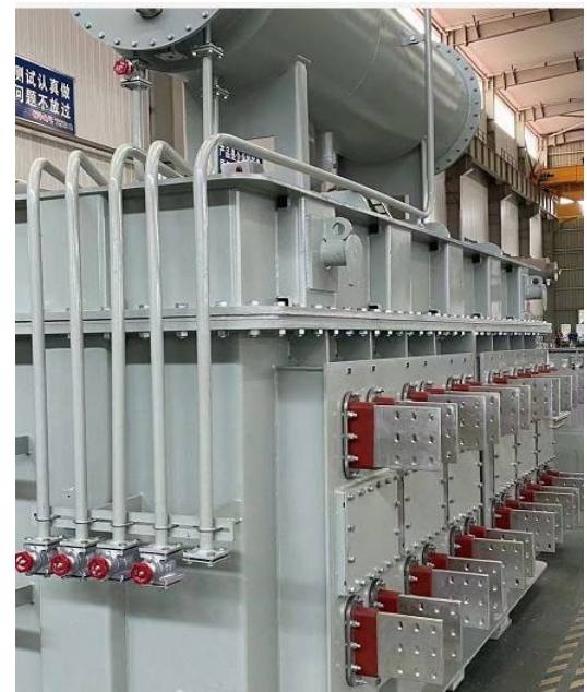
>110kV furnace transformer
