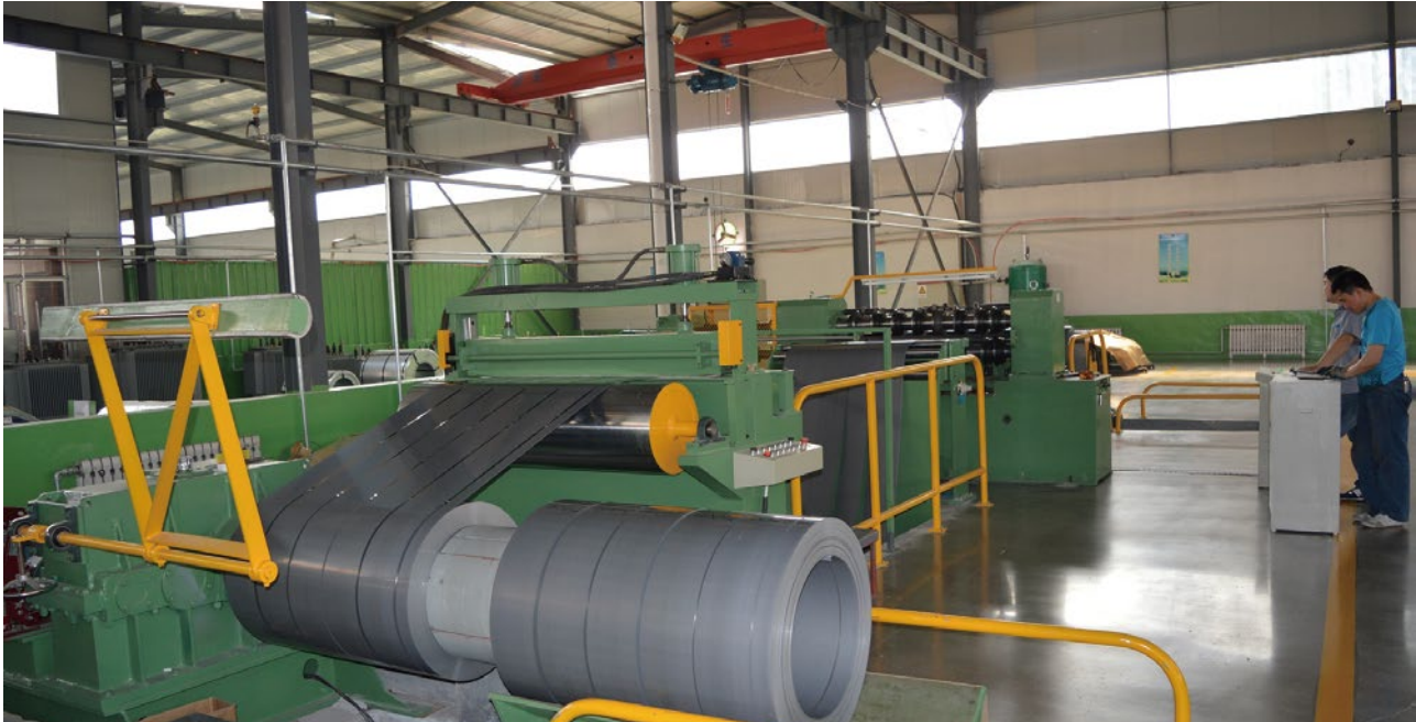
SILICON STEEL SHEET CROSSCUTTING MACHINE
