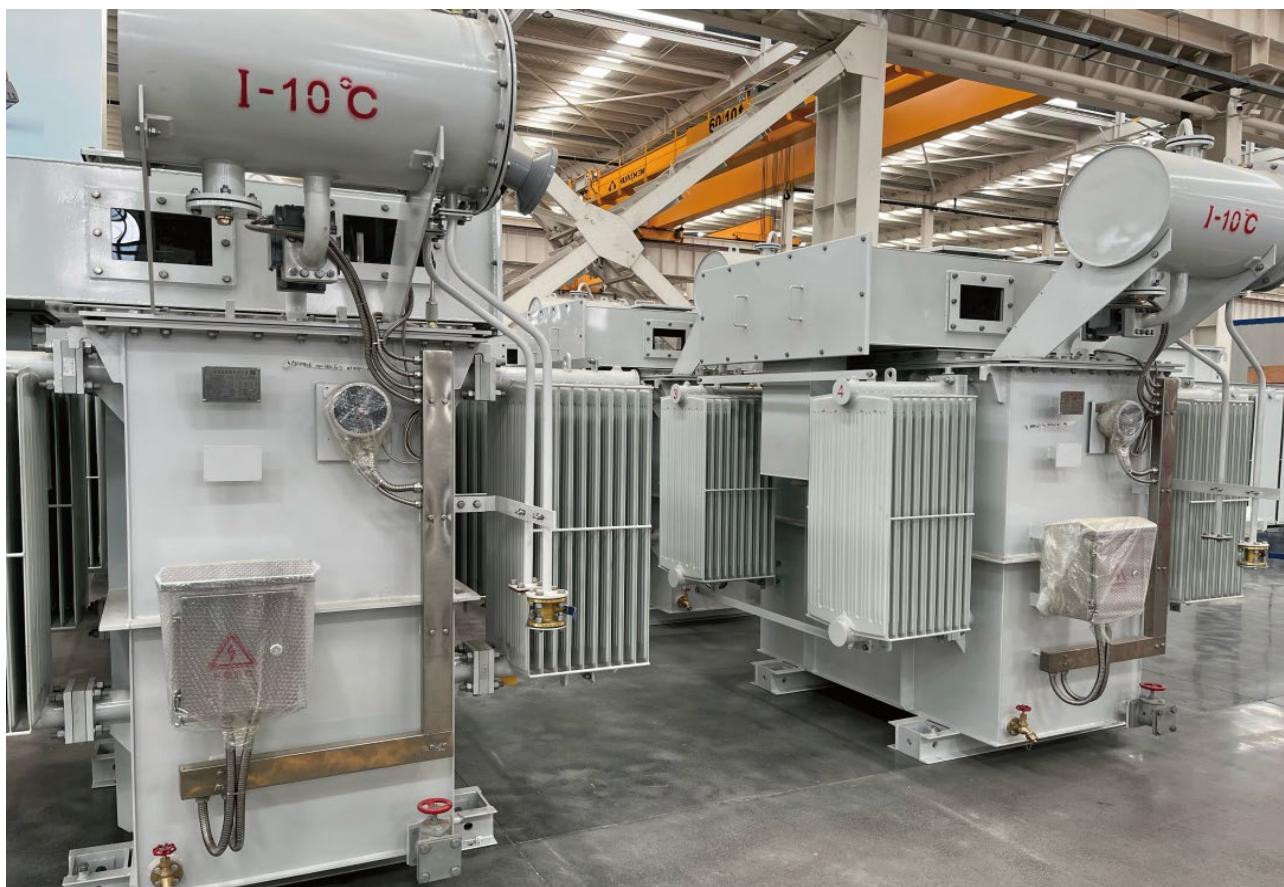
33kv-3150kva Oil immersed transformer
